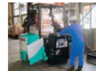
Changing the batteries of battery forklifts
