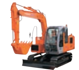
ZX70B, battery driven excavator
