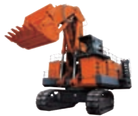
EX5500E-6, electrically driven ultra-large excavator
