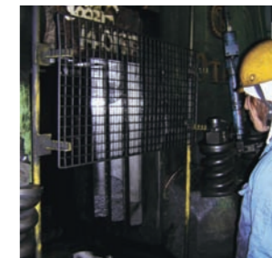
Press covered with a safety frame at Niigata Material
