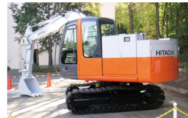
Electric power excavator
