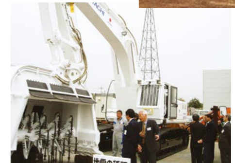
Flail hammer type demining machine
