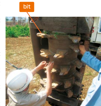
Rotating cutter of the landmine removal machine
