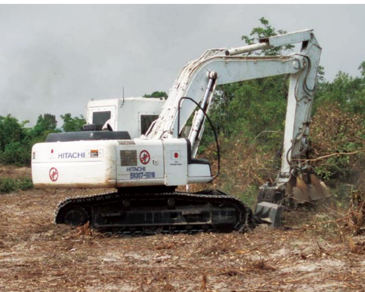
Demining machine in operation in Cambodia
