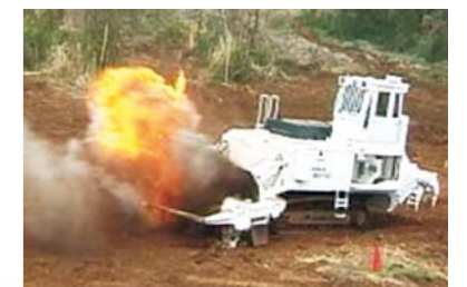
Demining machine in experiment using simulated landmines
